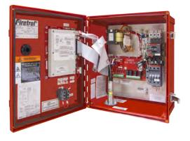
**Description**—Firetrol<sup>®</sup> FTA550F XG Jockey Pump Controllers are intended for use with fire pump systems. They are used for pressure maintenance in fire pump installations to prevent unnecessary operation of the main fire pump.
